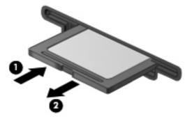
**NOTE:** If the card is not ejected, pull the card out of the slot.
